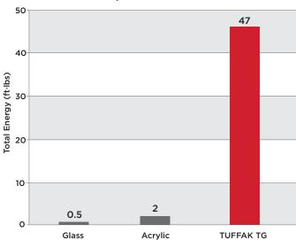
\*Instrumented Impact per ASTM D 3763, sample thickness is 0.125" nominal
