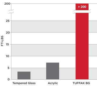
1/4" Thick Sheet - Steel Dart 1" Diameter Tip
