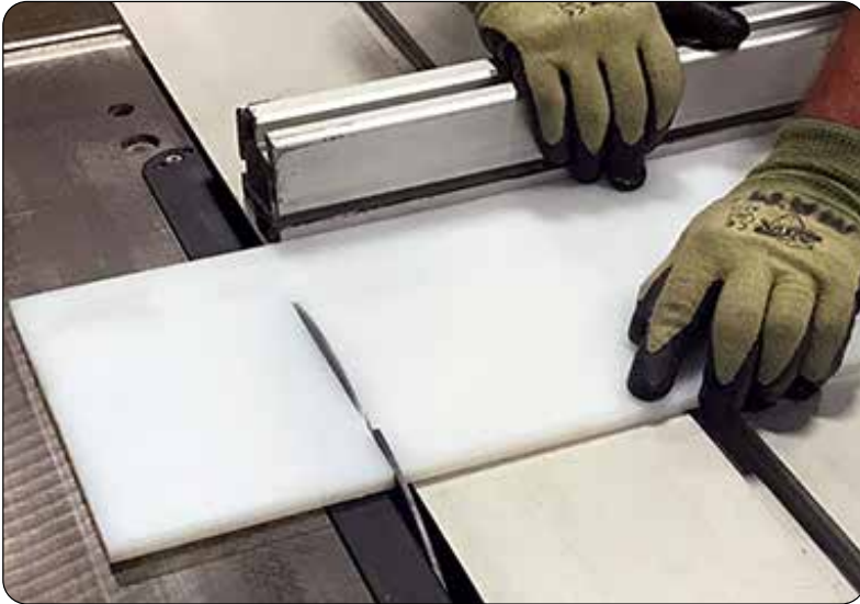
The "kerf" line can be seen in the above photo. Notice the faint line following the blade, that is the kerf line, where the blade cut through the sheet of plastic material.
