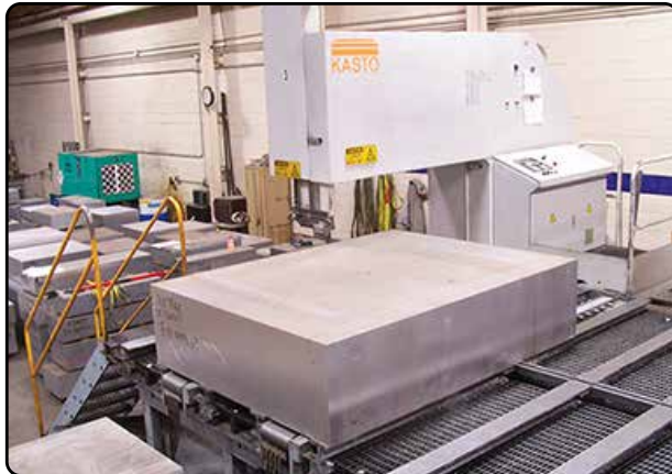
Alro has the capability to cut Aluminum Mold Plate up to 30" thick.
